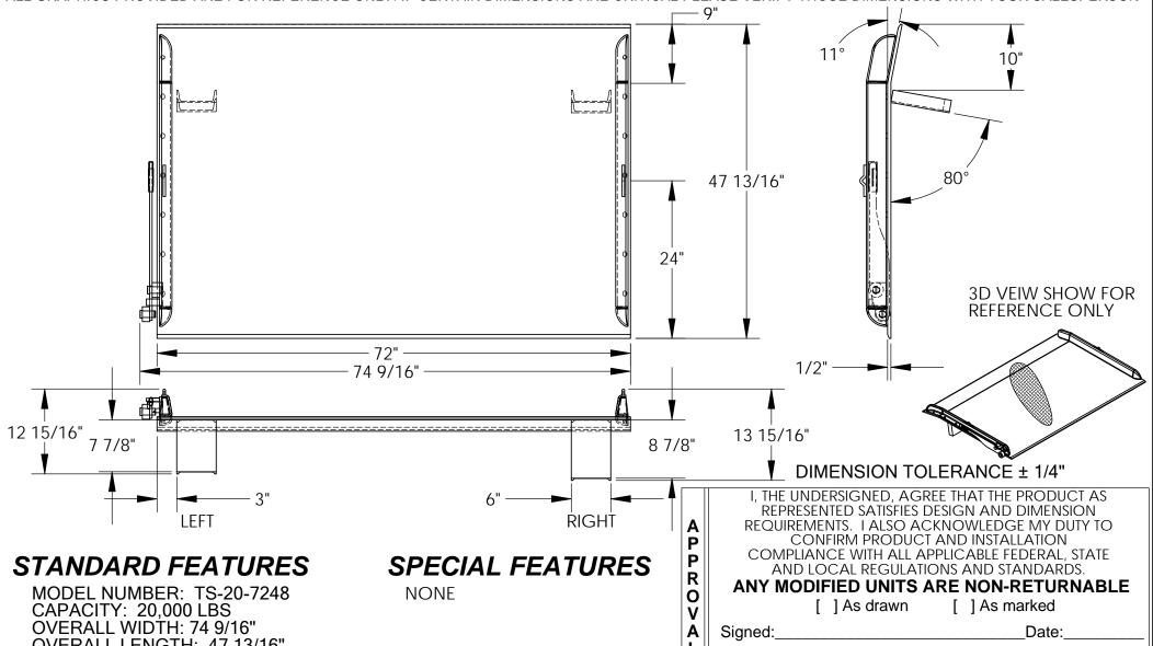
OVERALL LENGTH: 47 13/16" **DOCKPLATE THICKNESS: 1/2"** LEVER LIFT IS STANDARD LOCKING LEGS ARE 6" WIDE RIGHT LEG LENGTH IS 8 7/8" LEFT LEG LENGTH IS 7 7/8" CROWN IS 11° & 9" FROM EDGE **HEIGHT DIFFERENCE: 7"**
