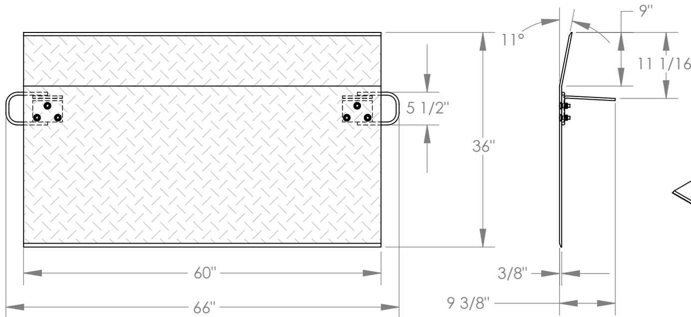
NOTE: BEND OR CROWN IS 11° AND LOCATED 9" FROM EDGE OF DOCKPLATE
